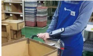
Routing instructions are sent to the device on the worker's arm
