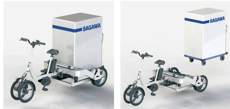
The towing section of the Trike Cargo vehicle attaches directly to a hand cart, and can be detached again with a single touch of a button (picture at right).
