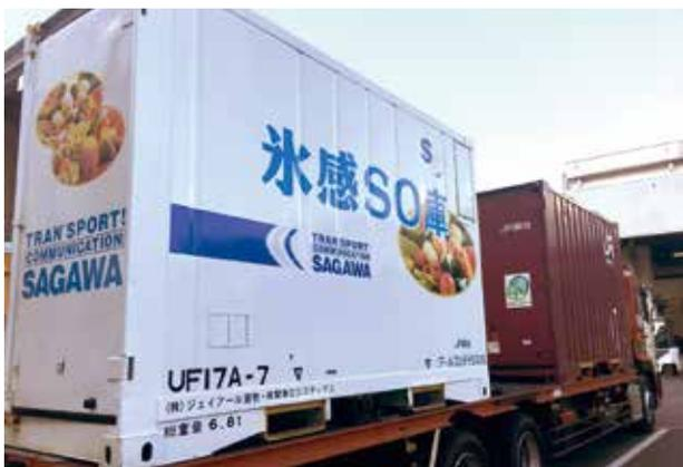
"Hyokan Soko" that manages a standard temperature via external power when stored and secondary battery power when in transport
